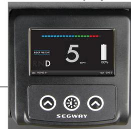
Provides operational data including speed, battery life and distance
